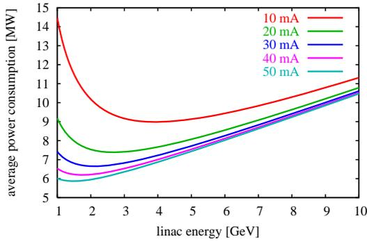
Figure 1: Av. SPL RF power at 50 Hz, 4 MW beam power for various pulse currents, top to bottom: 10 → 50 mA.
