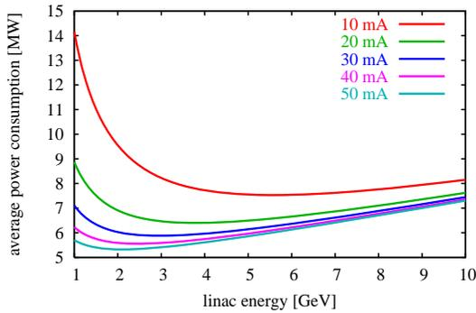
Figure 2: Av. SPL RF power at 25 Hz, 4 MW beam power for different pulse currents, top to bottom: 10 → 50 mA.
