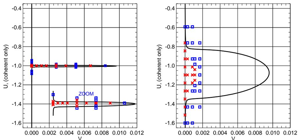
Figure 3: Comparison of results of simulations ( $\square$  and  $\times$ , see the previous figure for examples) with solution of the dispersion relation Eq. (2) (lines). Left: external nonlinearity alone, right: combination of external and internal (nonlinear space-charge) nonlinearities.  $V \propto \mathcal{R}e(Z^\perp)$ ;  $U \propto \mathcal{I}m(Z^\perp) \propto \Delta\Omega_{\text{coh}}$ .
