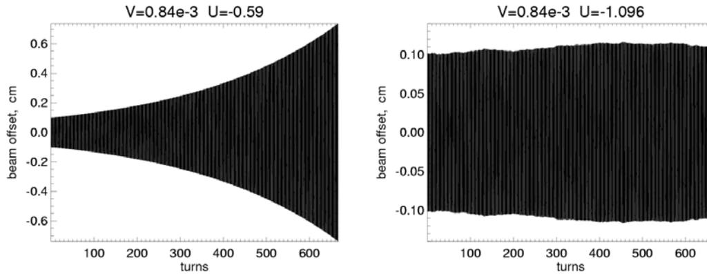
Figure 2: Typical time evolutions of the beam center from simulations using PATRIC for two different  $\mathcal{I}m(Z^\perp)$ ; left: no damping (instability); right: damping dominates (stable). Normalized impedances  $V, U$  correspond to Fig. 3, right.
