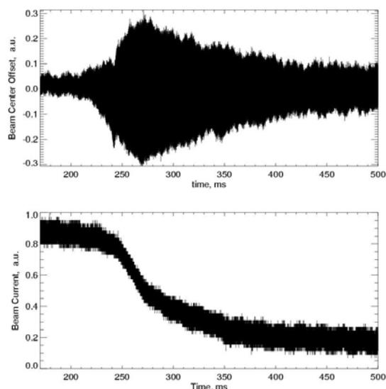
Figure 1: The transverse collective instability measured in SIS 18. Top: beam position, bottom: beam current.
