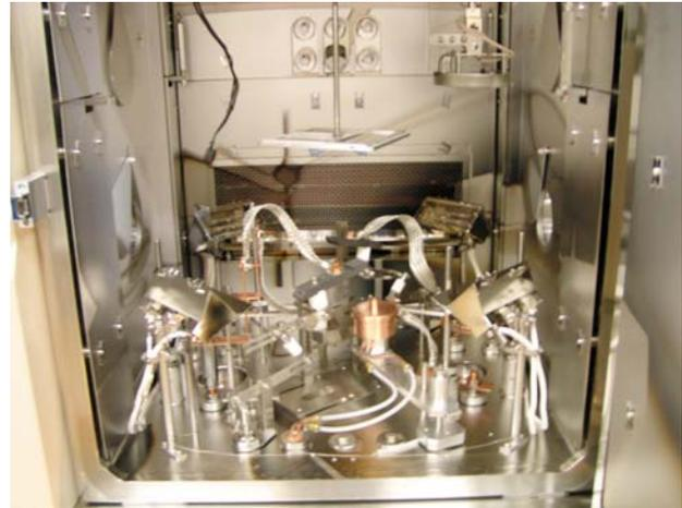
Fig.2 Arc-discharge evaporation-source in EBX-2000C cryo-vacuum pump apparatus
