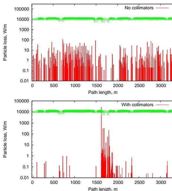
Figure 1: Beam loss distributions in Fermilab Main Injector at slip-stacking injection of 8-GeV protons without collimation (top) and with beam cleaning of 5% of beam intensity (bottom). (STRUCT calculations by A. Drozhdin).
