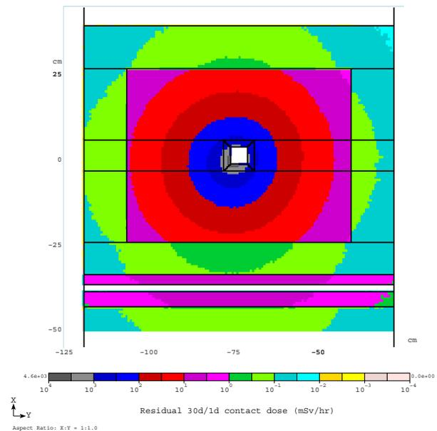
Figure 3: Residual dose transverse isocontours in the MI-8 collimator at longitudinal maximum after 30 days of irradiation at  $5 \times 10^{11}$  p/s and 1 day of cooling. The marble regions on the steel core outside are where the color is light-blue and green (less than a fraction of mSv/hr levels).
