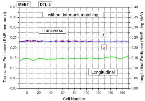
Figure 8. Transverse and longitudinal emittances.
