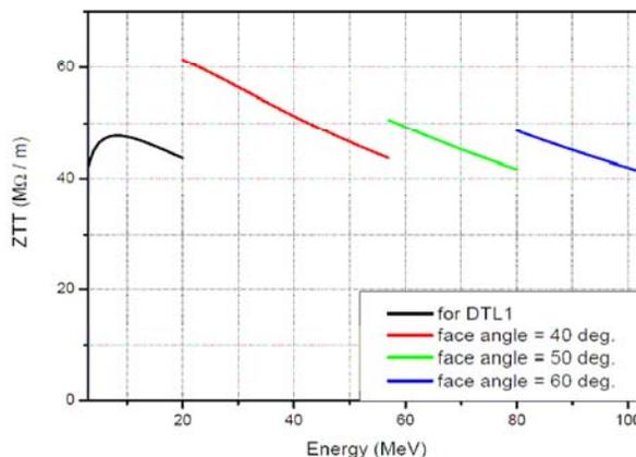
Figure 1. Effective shunt impedance per unit length depending on energy.
