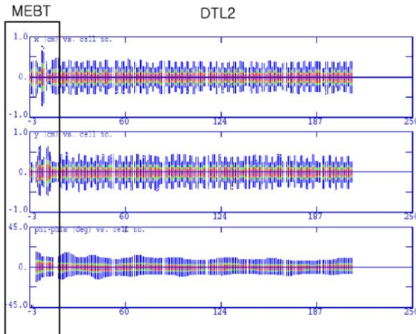
Figure 5. Configuration plot of the 20 mA proton beams in PEFP MEBT and DTL2.
