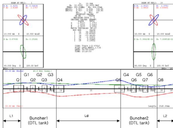
Figure 2. TRACE3D matching between DTL1 output beam and DTL2 input beam using MEBT.
