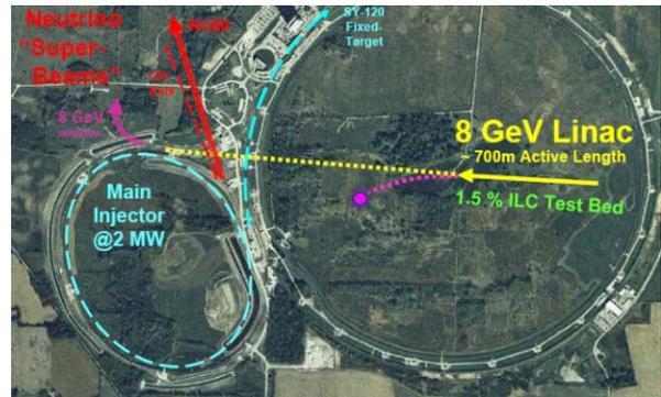
Figure 10: Fermilab 8 GeV SCRF linac layout.
