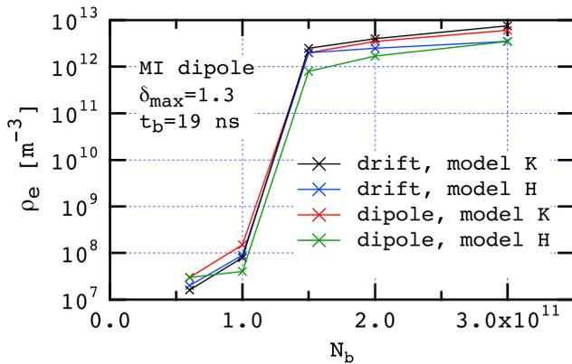
Figure 3: Average electron density in steady state for the MI vs.  $N_b$  assuming  $\delta_{\max} = 1.3$ . This choice for  $\delta_{\max}$  is meant only as an initial step in a more comprehensive analysis yet to be carried out. Models “H” and “K” represent two choices for certain details of the SEES. Model “H” for the MI is the same as model “R” for the LHC (Fig. 2).
