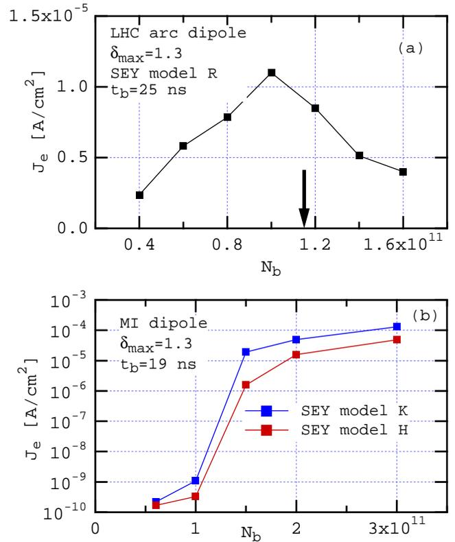
Figure 5: Average electron flux at the wall for the choice  $\delta_{\max} = 1.3$ . (a) LHC arc dipole magnet at beam energy  $E_b = 7 \text{ TeV}$ ; (b) MI dipole at  $E_b = 8 \text{ GeV}$ . The models refer to specific parameter choices for the SEY and SEES. Model “K” for the MI is the same as model “R” for the LHC. The arrow in (a) indicates the nominal bunch intensity,  $1.15 \times 10^{11}$ .
