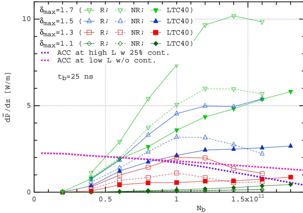
Figure 1: Average power deposition per unit length of chamber in an LHC arc dipole magnet vs.  $N_b$  for  $t_b = 25$  ns. “R:” full SEES; “NR:” SEES without the rediffused component; “LTC40:” results from Ref. 9; “ACC:” available cooling capacity of the cryogenic system at high luminosity with 25% contingency, or at low luminosity with no contingency.
