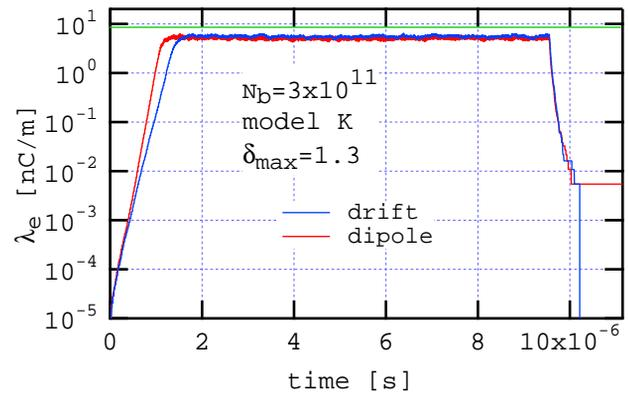
Figure 4: Build-up of the average EC line density during one revolution in the MI for  $N_b = 3 \times 10^{11}$ . The horizontal green line represents the average beam neutralization level, given by  $\lambda_b = eN_b/s_b = 8.5$  nC/m, where  $s_b = 5.6$  m is the bunch spacing (or RF wavelength, in this particular case).
