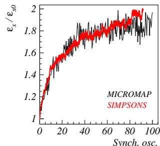
Figure 8: Emittance evolution for the full bunch.
