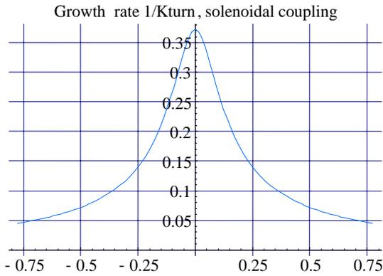
Fig. 1: Ion-electron growth rate, in inverse Kturns ( $10^{-3}/T_0$ ) as a function of the tune separation  $\mu_x - \mu_y$ , reproducing Fig. 1 of Ref. [11].
