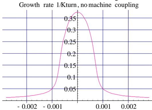
Fig. 2: Growth rate plot similar to Fig. 1, except the solenoid coupling is compensated. The peak maximum is the same, but the width is reduced  $\sim 300$  times.
