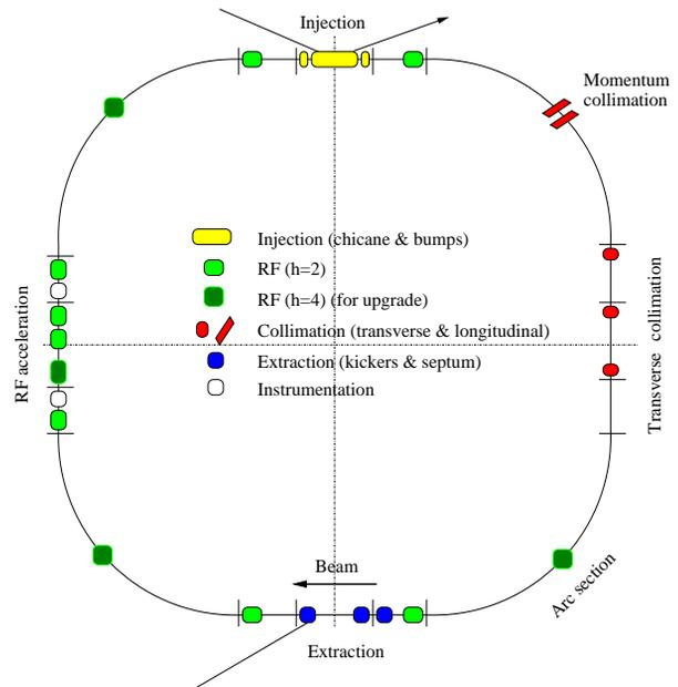
Figure 3: Schematic layout of the CSNS synchrotron.
