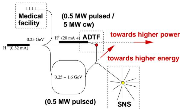
Figure 8: Possible CSNS upgrades towards higher power, higher energy, and multipurpose.
