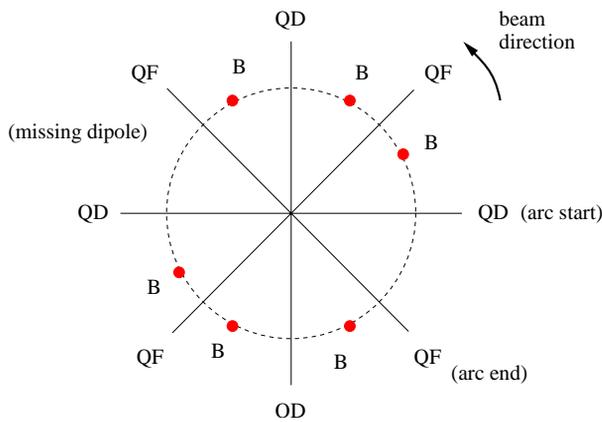
Figure 5: Dispersion suppression with a single missing dipole shown in the horizontal phase space.
