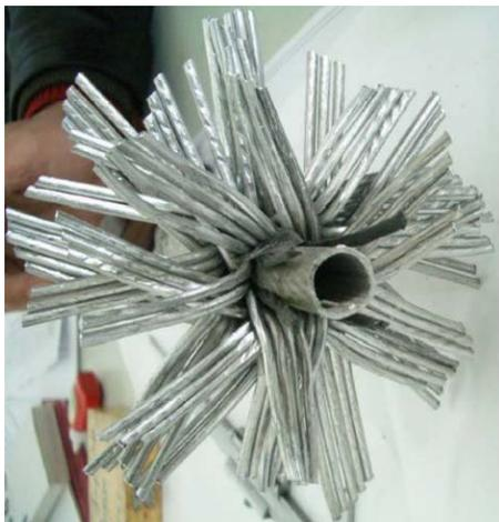
Figure 6: One of the first prototypes of the J-PARC type braided magnet coil fabricated by a vendor in China.
