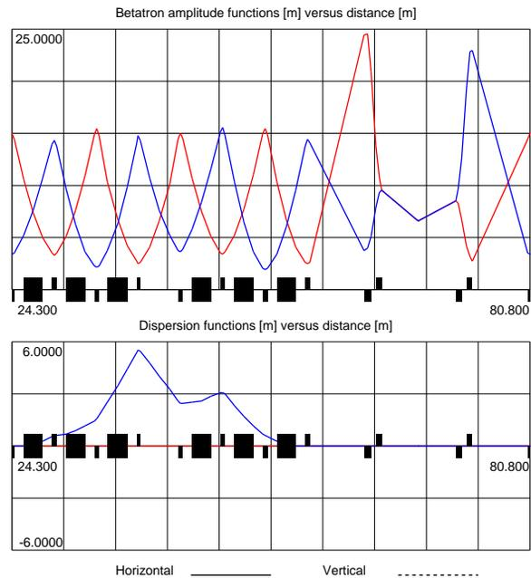
Figure 4: CSNS synchrotron lattice functions in one super-period. The ring has a periodicity of 4.
