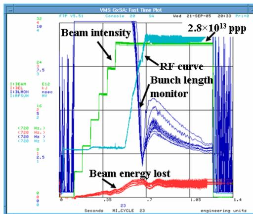
Figure 5: ‘NuMI only’ cycle in Main Injector
