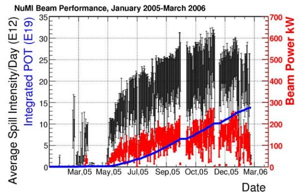
Figure 7: Spill intensity, beam power and integrated protons on target for the first year of NuMI operation.
