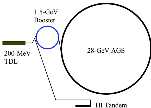
Figure 2 The AGS Accelerator Complex
