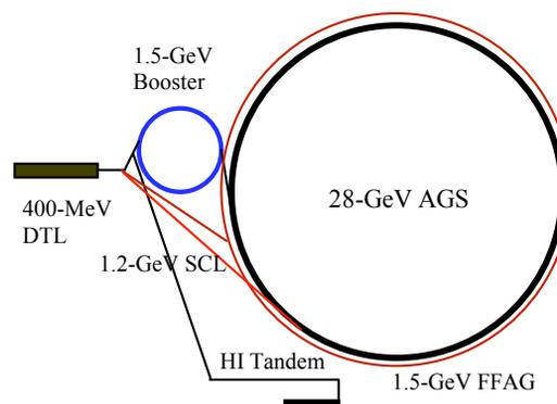
Figure 3. AGS Upgrade with a 1.2-GeV SCL or a 1.5-GeV FFAG in the AGS Tunnel
