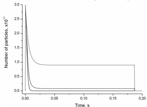
Figure 6: Expected  $U^{28+}$ -beam intensity evolution in SIS18 during a 4 Hz booster sequence, calculated with StrahlSim. It was assumed that only 8 % of the gases desorbed inside the “desorption” scrapers are able to interact with the revolving beam. The different curves indicate different steps of the UHV system upgrade.
