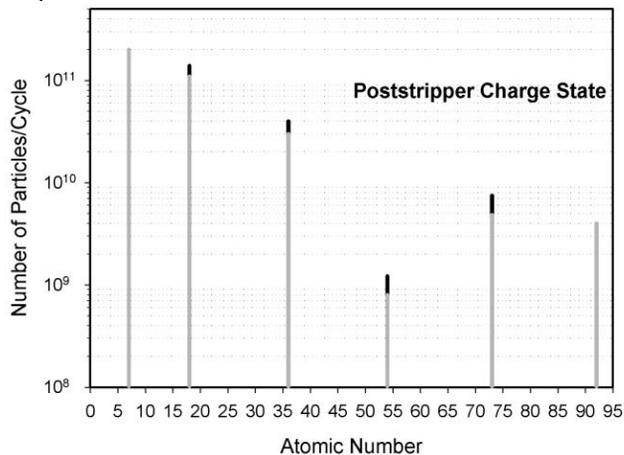
Figure 5: Present status of maximum number of particles of ions with different atomic numbers and intermediate charge states accelerated in SIS18.
