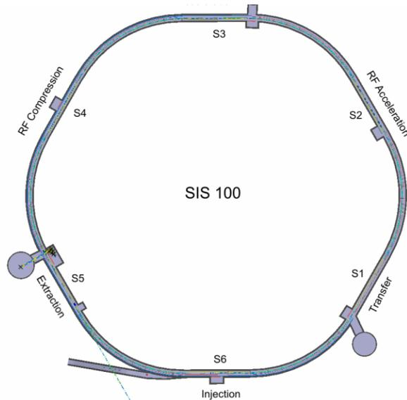
Figure 2: Distribution of the injection-, extraction- and transfer systems and the RF systems for acceleration and bunch compression in the six straight sections of SIS100
