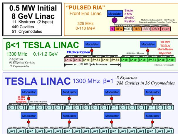
Figure 5: Layout of FNAL Proton Driver.
