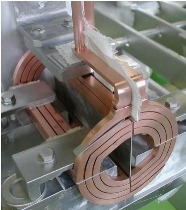
Figure 7: Electromagnetic coil produced with the electroforming technique and the wire-cutting. Water cooling channels therein.
