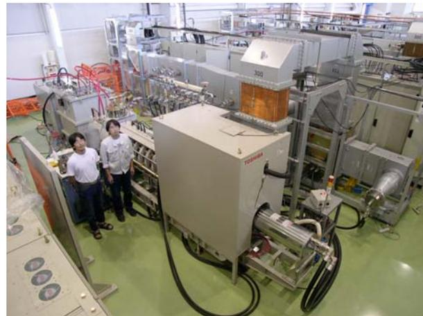
Figure 8: 324-MHz, 3-MW klystron with a repetition of 50 Hz and a pulse length of 600  $\mu$ s
