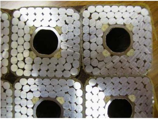
Figure 5: The cut-away view of the stranded coil used for the bending magnet
