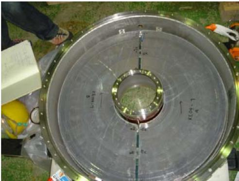
Figure 6: Cut MA cores for the J-PARC
