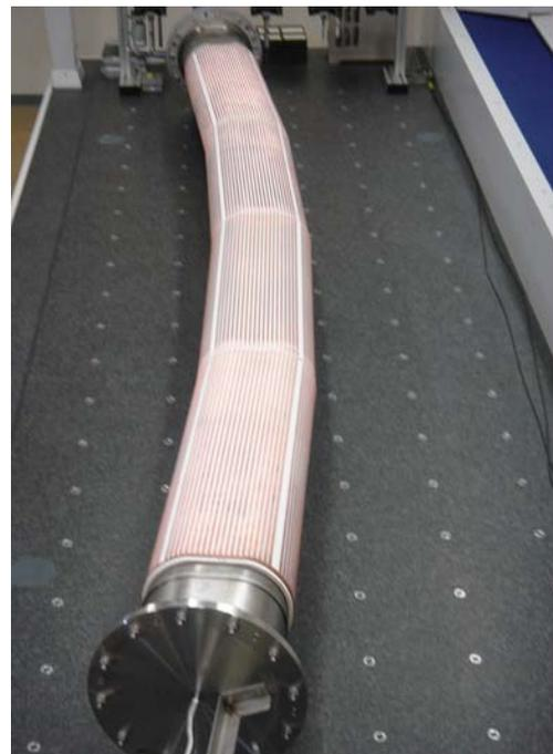
Figure 4: The ceramics vacuum chamber for the J-PARC RCS bending magnets
