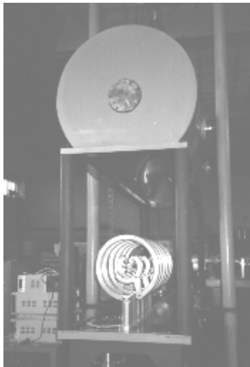
Fig. 6 The Cavity tank of 1 MeV RFQ
