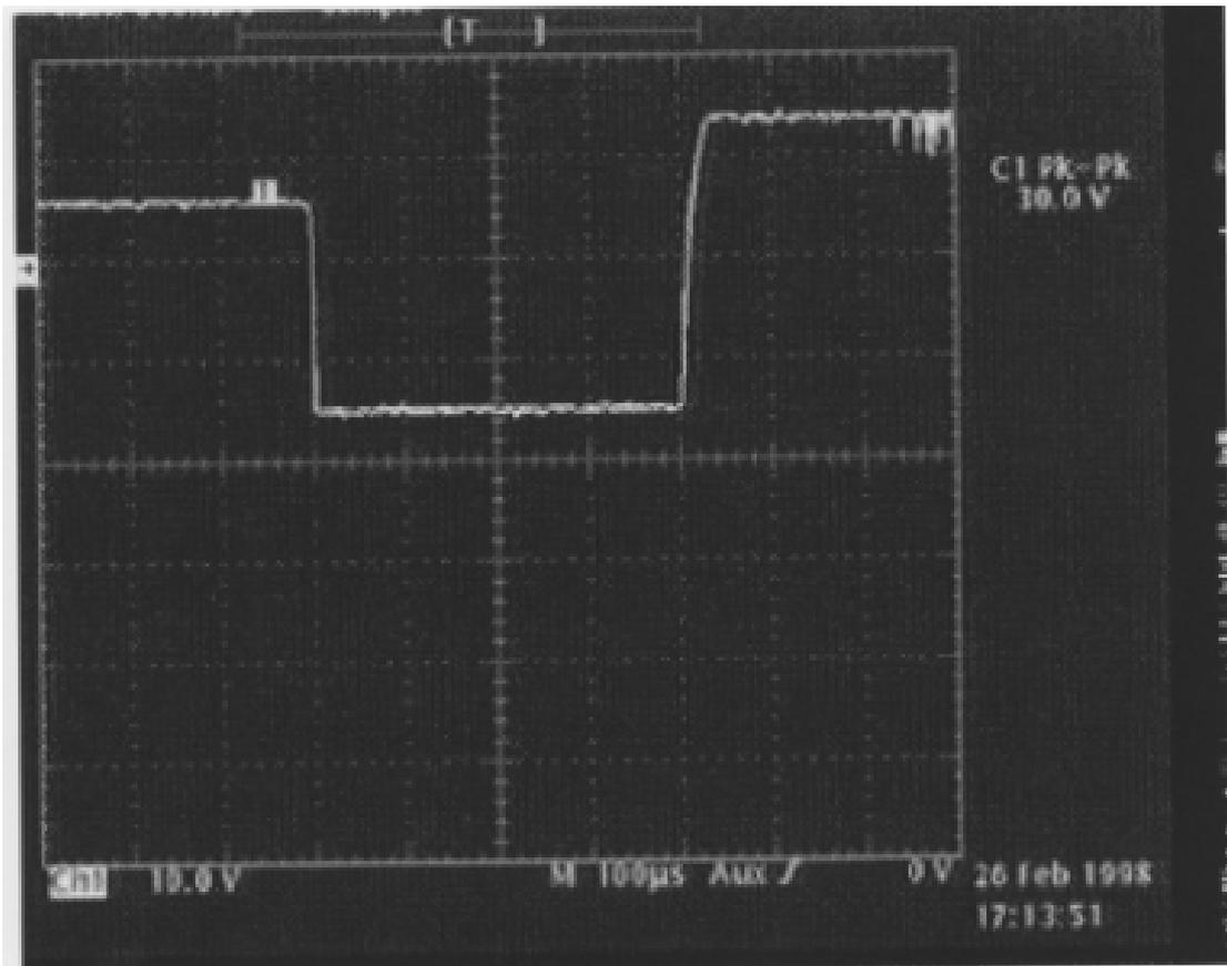
Fig.1, Stable oscillation in the wavelength of around  $24 \mu\text{m}$  has been observed by using the Ge(Cu) detectors and home-made fast current amplifier system. Macropulse width is about 0.4ms, beam current ranging from 2 to 4mA, and laser power of several tens watts in average.
