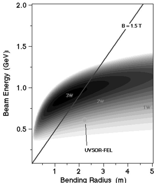
Figure 3: Contour plot of the intracavity power for 200 nm FEL. The cavity loss of 4% is assumed. The solid line shows the border between field strengths of normal conducting magnets and superconducting magnets.
