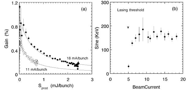
Figure 2: The deduced FEL gain as a function of the total extracted photon energy (a). Saturation energies for one electron at various beam current (b).
