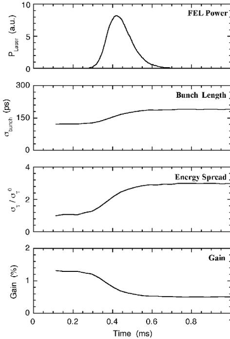
Figure 1: The FEL power and the electron bunch evolutions in a Gain switching lasing. The bunch distribution was observed by a dual-sweep streak camera, and the energy spread was deduced by taking a potential-well distortion into account.
