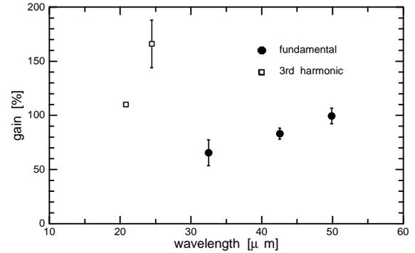
Figure 2: FEL gain as a function of the wavelength below 50  $\mu\text{m}$ . The data points denoted by the filled circles and the open squares are assigned to the fundamental oscillation and third harmonic oscillation, respectively.
