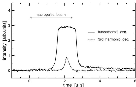
Figure 4: The time spectra of the laser light from the FEL operated at a wavelength of 164  $\mu\text{m}$  measured with the fast Ge:Ga detector. The solid and the dotted lines are for the fundamental and the third harmonic oscillations, respectively. Saturation of the FEL signal for the fundamental oscillation is not that of the FEL oscillation but that of the detector.
