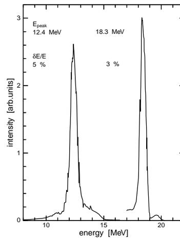
Figure 1: The energy spectra of the electron beam from the L-band linac.
