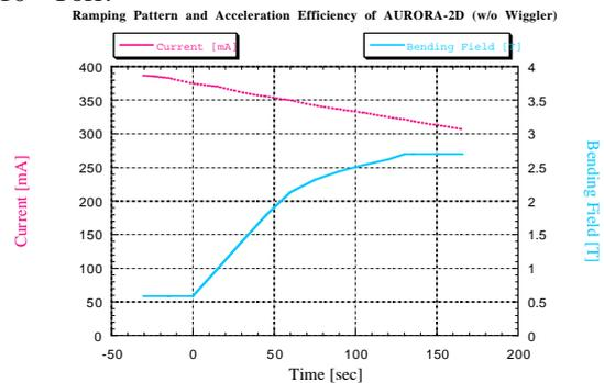
Fig. 4-a) Typical acceleration pattern of A2D.
