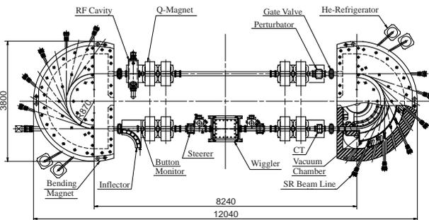
Fig. 2-b) Plan of A2D with 7 Tesla wiggler.
