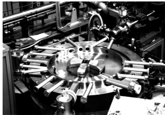
Fig. 3 Inside of the vaccum chamber is shown. Pair of the perturbator and dual accelerator cavitys are seen. Every component has a slit of 12 mm wide in the median plane.
