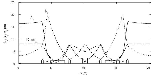
Fig. 5. Betatron functions and the dispersion in the small emittance operation mode.
