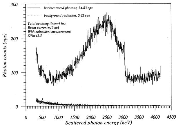
FIG. 2  $\gamma$ -ray spectrum of Compton scattering with collimator of  $3\text{mm}$  diameter under synchronous measurement. (electron beam current= $19\text{mA}$ , counting time= $4\text{hrs.}$ , and  $S/N$  ratio = $42.5$ .)
