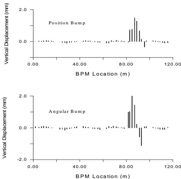
Fig. 3 A typical orbit position bump (upper one) and a typical orbit angular bump (lower one).
