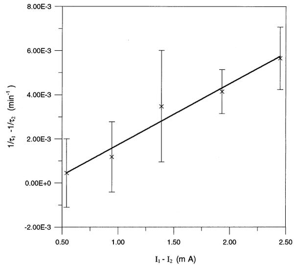
Fig. 5 The Touschek lifetime measurement by the two unequal bunch beam method. The horizontal axis is the difference between the two bunch currents in units of mA. The vertical axis is the difference of the inverse of the bunch total lifetime.
