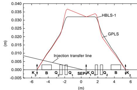
Fig. 9(a) Sketch map of existing three-kicker system and bump orbits of GPLS, HBL
