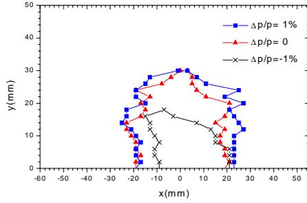
Fig. 5 Dynamic aperture with fourteen sextupoles
