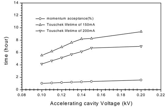
Fig. 11 Lifetime vs. RF cavity voltage
