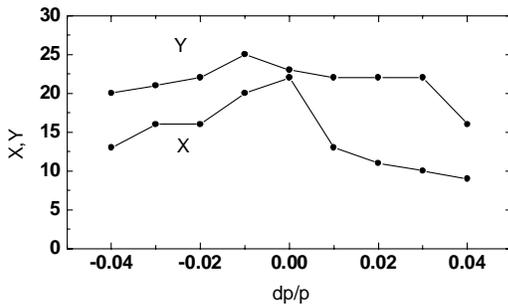
Figure 5 Dynamic apertures vs. energy deviation at the mid-point of the super-long straight section.
