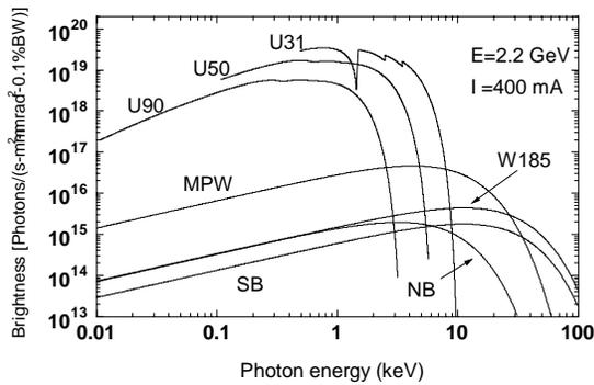
Figure 6 Brightness of radiation generated at SSRF
