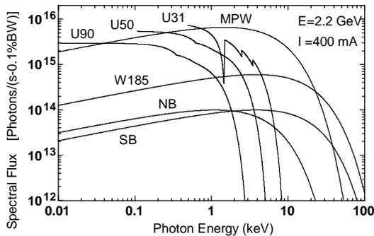
Figure 7 Spectral flux of radiation generated at SSRF
