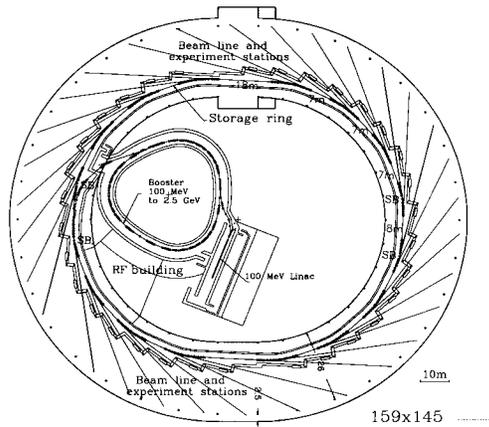
Figure 1 Layout of the SSRF
