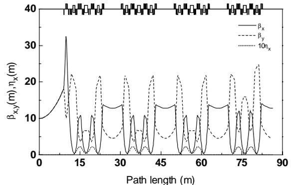
Figure 2 Lattice functions of one quarter of storage ring
