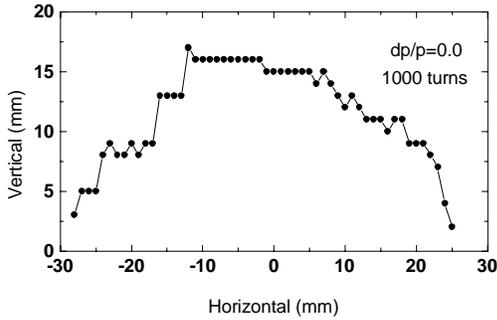
Figure 3 Dynamic aperture at the injection point
