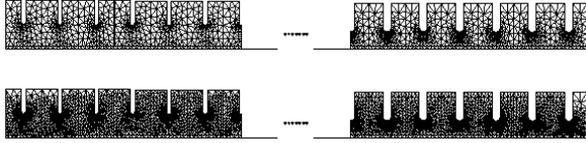
Figure 3: Adaptive mesh refinement of 206 cell section on parallel computer using Omega2P.
