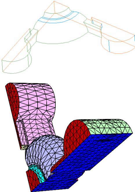
Figure 4: DDS cell: solid model (top), finite element mesh (bottom) as computed with Omega3.
