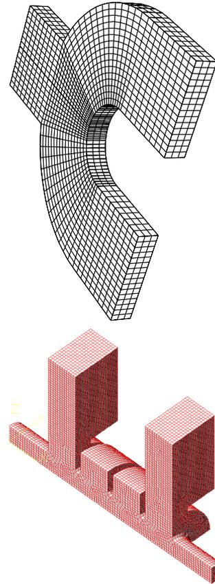
Figure 5: Tau3 modeling of bifurcated waveguide feed and power input coupler to accelerator structure.
