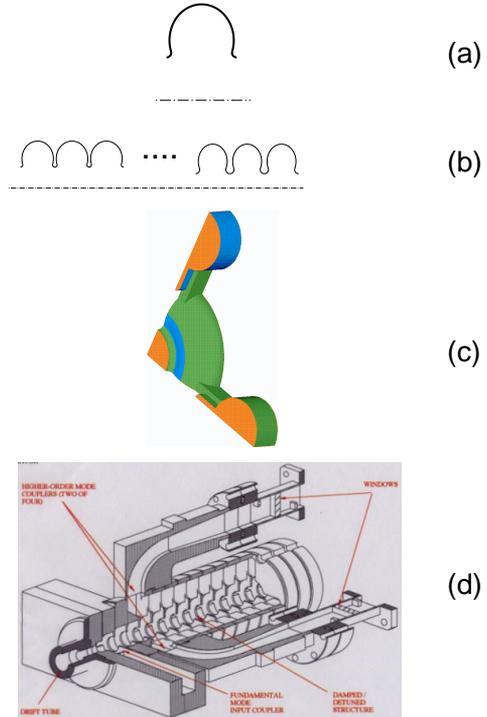
Figure 1: (a) Optimized, detuned cell design (Omega2), (b) Detuned structure of 206 cells wakefield analysis (Omega2P), (c) Damped, detuned cell design (Omega3), (d) Damped, detuned structure (Omega3P)
