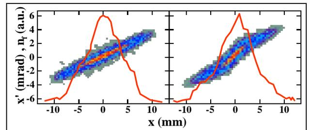
*Figure 1: Phase-space distribution and profile measured in front of the FODO channel at beam currents of 2.2 mA (left) and 37 mA (right).*
