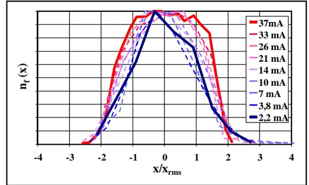
**Figure 3:** Measured beam profiles at the FODO-channel exit.
