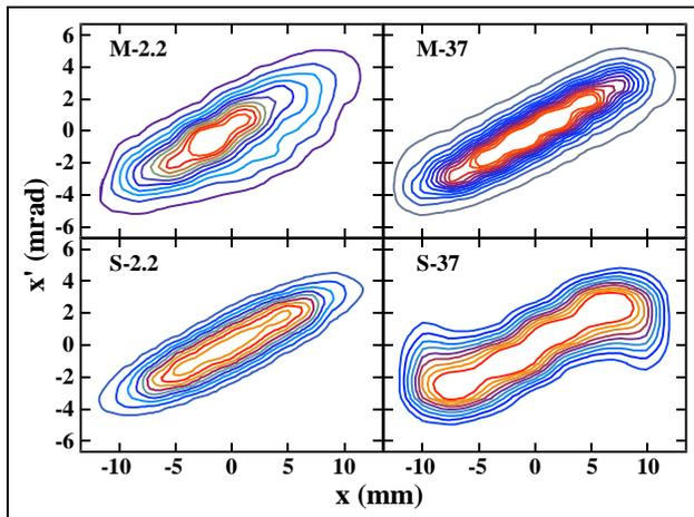
**Figure 2:** Comparison of measured (above) and simulated (below) phase-space contour plots for beam currents of 2.2 mA (left) and 37 mA (right).
