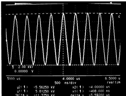
Figure: 1 Obtained RF voltage by a test cavity in which one FINEMET core was installed.
