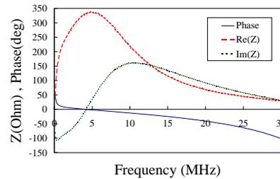
Figure 3: Impedance of the HG cavity.
