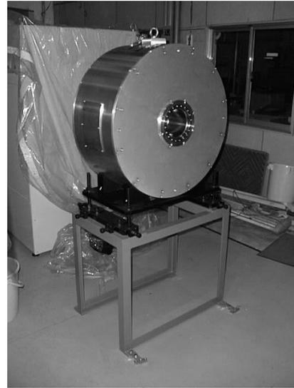
Figure: 2 High Gradient RF cavity. A 200 kW class push pull amplifier will be located under the cavity.
