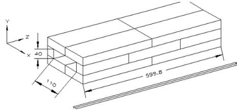
Figure 4: Structure of kicker magnet core.
