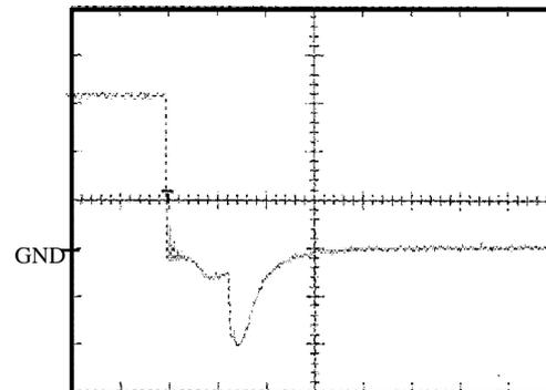
Figure 3: Thyatron anode voltage (16 kV charging) (5V/Div., 2 $\mu s$ /Div.). 1kV/V, 16kV peak
