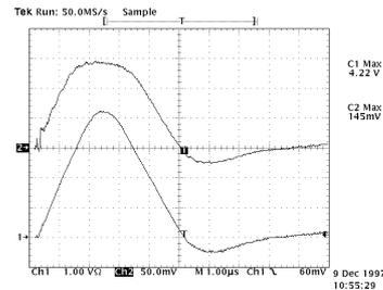
Figure 7: Waveforms of current(bottom: I=16.4 kA) and magnetic flux density(top) at point B in Fig 6.
