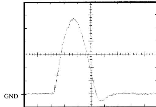
Figure 2: Measured load current (16 kV charging) (2 V/Div., 2  $\mu s$ /Div.). 2kA/V, 22.8 kA peak, 6.32  $\mu s$  pulse-width, 4.08  $\mu s$  FWHM.
