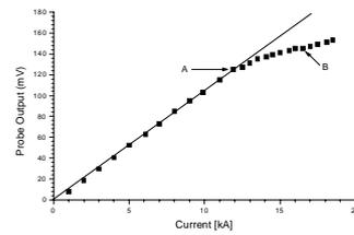
Figure 6: Peak current versus peak magnetic flux density in the kicker magnet.
