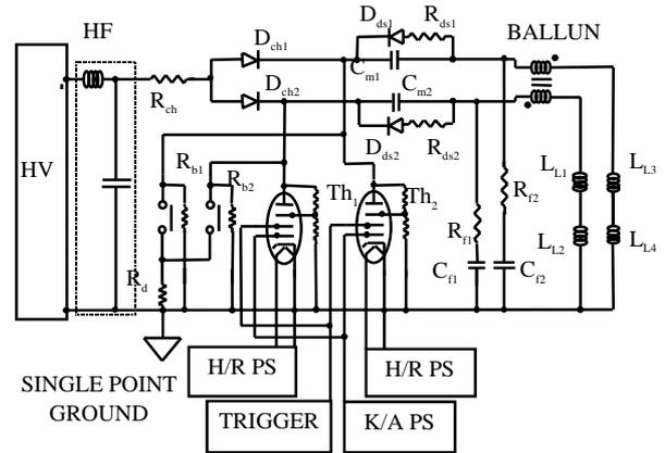
Figure 1: Schematic Circuit Diagram of Kicker Magnet Modulator.
