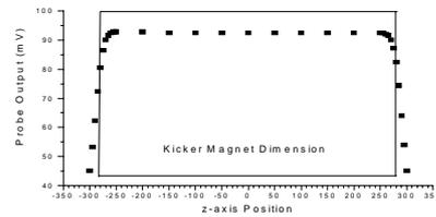
Figure 5: Z-direction spatial field distribution in kicker magnet.
