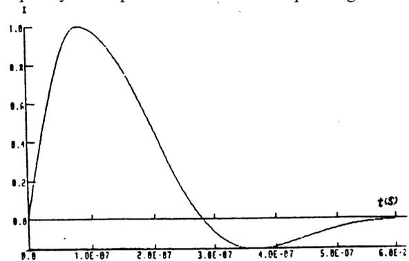
Fig.1 A optimized driving current waveform
