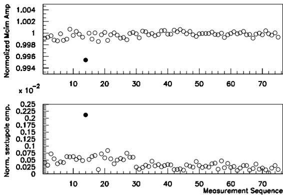
Figure 3: The main amplitude and the normalized sextupole component are plotted against the magnet measurement sequence. The solid circle in each plot (the 14th magnet to be measured) corresponds to the short-layered magnet.
