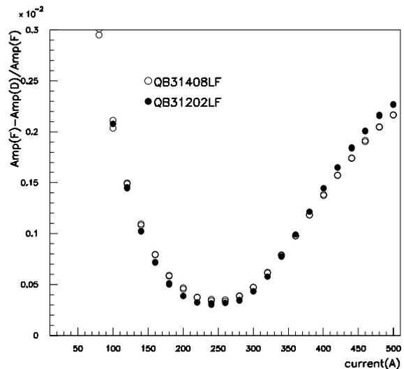
Figure 6: The main amplitude difference between the F- and D-connections is plotted as a function of current for two TRISTAN F-type magnets. The hysteresis effect has a minimum at around 250A.
