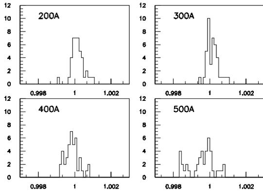
Figure 4: Qrf(LER) main quadrupole amplitude distribution at various currents. Three groups appear at 500A due to iron permeability differences.
