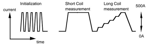
Figure 2: A typical scenario for series measurements.
