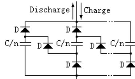
Fig. 2: Diagram of Discharge /Charge of  $n (C/n)$  s in Series/Parallel
