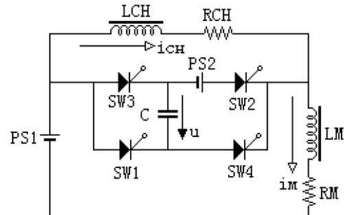
Fig.1. Fundamental Principle of the SRMPS
