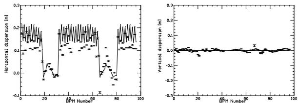
Figure 4: (Left) horizontal and (right) vertical dispersion; measurement (symbols) and model (lines).
