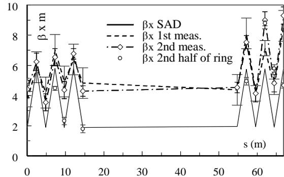
Figure 2: Local  $\beta_x$  measurements at QF2R quadrupoles.
