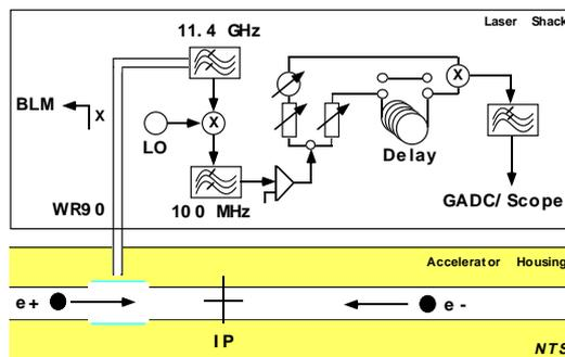
Figure 1: Schematic of BTM signal processing.
