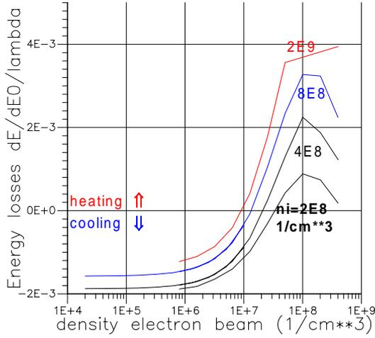
Figure 4: The losses energy of ion beam after passing cooling section: if losses negative it means cooling, if positive it means heating.
