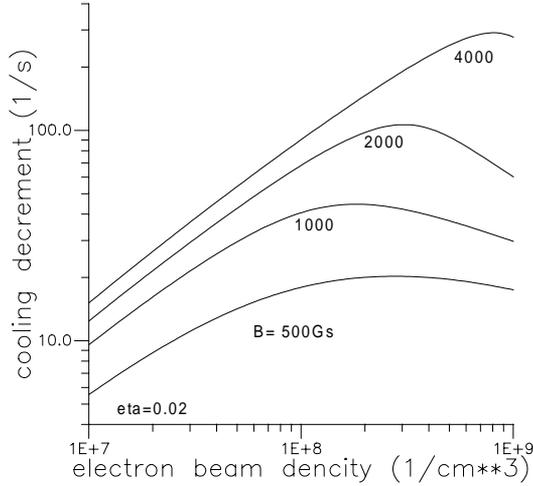
Figure 1: The cooling rate for different solenoid fields, 0.5,1,2,4 kGs.
