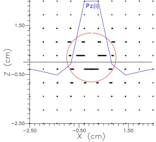
Figure 2: The crosssection of ion beam after passing cooling section. The circular show region of fluctuation, the points the position of electrons, the line distribution of the transverse momentum by action of electric field.
