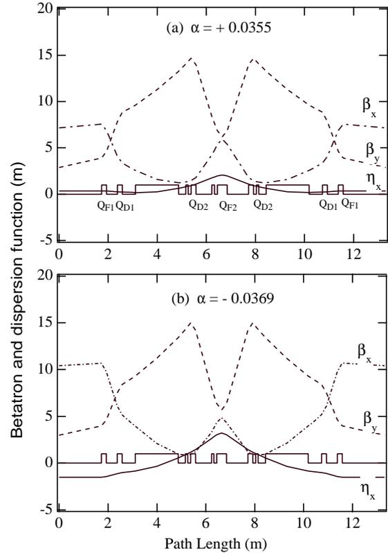
Fig. 1 Calculated Twiss parameters for one unit cell as positive  $\alpha$  (a) and negative  $\alpha$  (b) operation.
