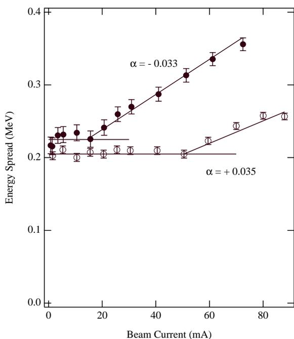
Fig. 3 Beam current dependence of the energy spread derived from the modulation factor of radiation spectra from the optical klystron. Lines are guided by eyes.
