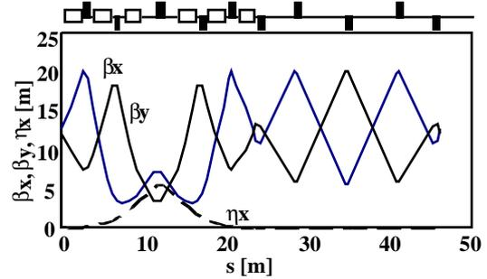
Fig. 3(a) Beta function and dispersion function of the 20 cell FBDO lattice
