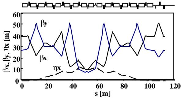
Fig. 2 Magnet lattice for the achromat region in the HEBT
