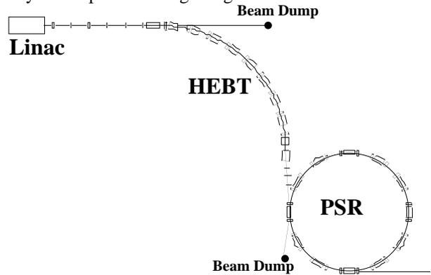
Fig. 1 Layout of the proton storage ring
