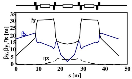
Fig. 3(b) Beta function and dispersion function of the Triple Bend Achromatic lattice
