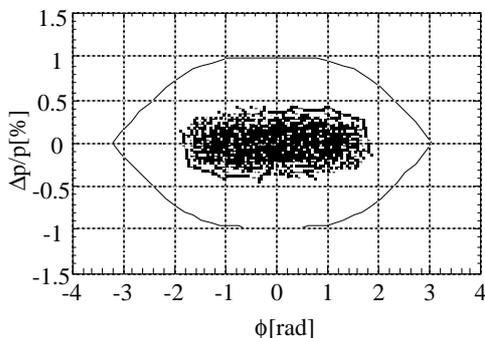
Fig. 4 Beam distribution in a longitudinal phase space
