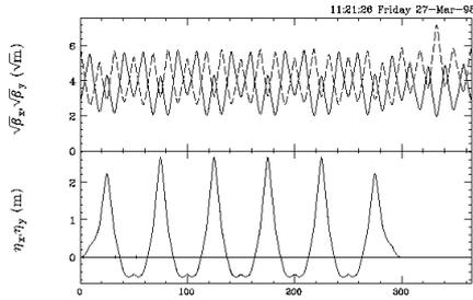
Figure: 2 Lattice functions with dispersion suppressor.
