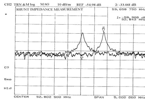
Fig.5- Setup and Results of Frequency Shift Method for the Measurement of Shunt Impedance MHz.
