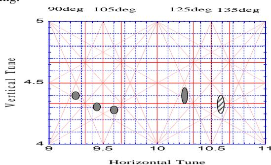
**Figure 4.** Tune Diagram. We could store 400 mA beam at the shaded area with dots. We could store a few mA beam at the shaded area with lines, without the sextupoles but still cannot inject with the sextupoles on.
