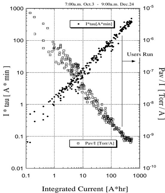
**Figure 2.** The result of vacuum conditioning. The black circles are the lifetime multiplied by the beam current. The white squares are the average pressure normalized by the beam current. The horizontal axis is the integrated current as a measure of time. The data from Oct. 1 to the end of 1997 are shown. The start of the users operation is indicated in the figure.
