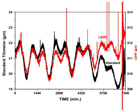
Figure 5: Ground motion in the quiet granite tunnel. The data are taken at the same position, but using different methods. Both sensors are separated by a distance 28 m.
