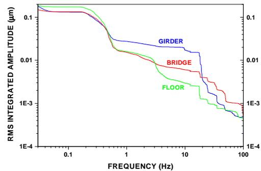
Figure 4: Horizontal vibration in the experimental hall of KEKB.
