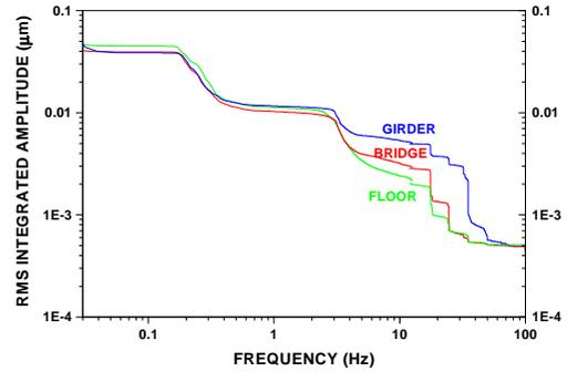
Figure 3: Integrated vertical vibration in the experimental hall of KEKB. BRIDGE is a construction on the floor and GIRDER is set up for the final focus magnet.
