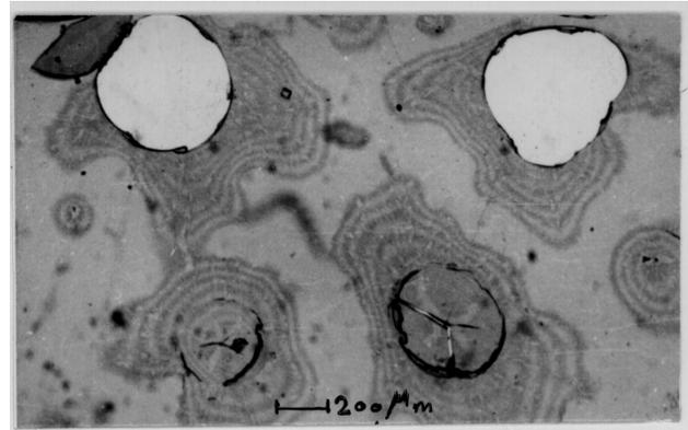
Fig 5. Electron Beam spots on Target Surface
