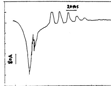
Fig 1. pseudospark pulsed electron beam current wave
