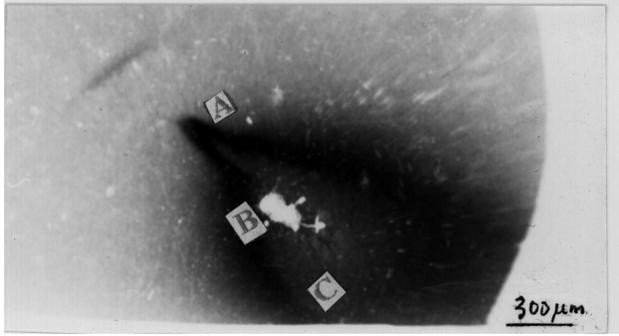
Fig. 3. Pulsed electron beam after deflection cross the magnetic field (A) high energy point, (B) Center region, (C) low energy region
