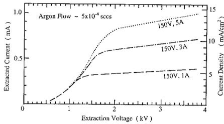
Fig. 2. Child-Langmuir curves for Argon beam at 3 power levels.
