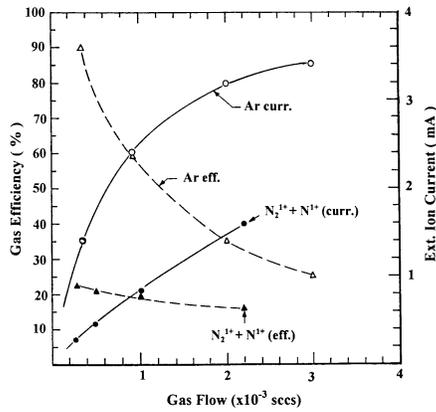
Fig. 3. Source gas efficiency as a function of flow at 0.5 kW.
