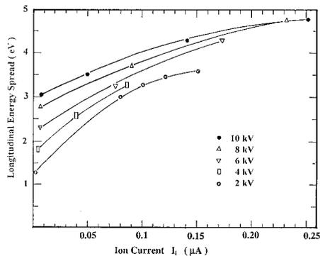
Fig. 4. Energy spread as a function of beam energy and  $I_i$ .
