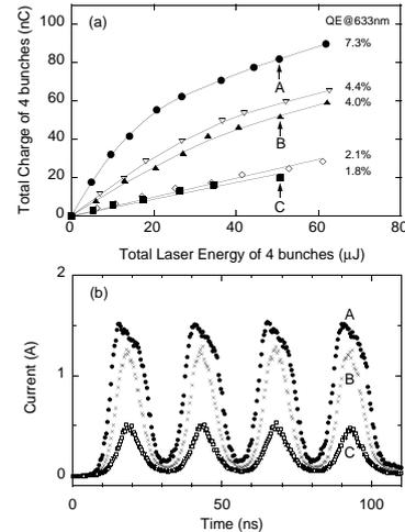
Fig. 4. Charge saturation behaviors taken for different QE states for a GaAs-AlGaAs superlattice with a high surface doping of  $4 \times 10^{19} \text{ cm}^{-3}$  (SL-1 sample).
