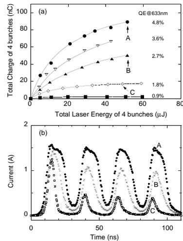
Fig. 5. Charge saturation behaviors taken for different QE states for a GaAs-AlGaAs superlattice with a medium surface doping of  $5 \times 10^{18} \text{ cm}^{-3}$  (SL-2 sample).
