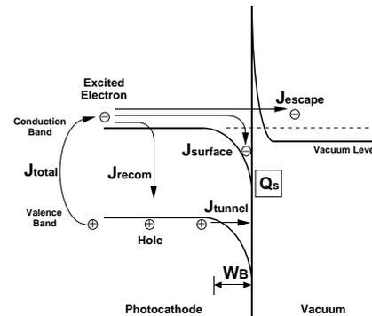
Fig. 1 Photoemission process for an NEA photocathode.
