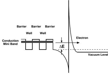
Fig. 2. Energy diagram of a conduction mini-band in an NEA superlattice.
