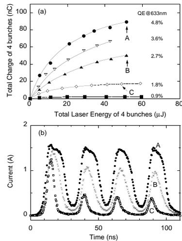
Fig. 5. Charge saturation behaviors taken for different QE states for a GaAs-AlGaAs superlattice with a medium surface doping of  $5 \times 10^{18} \text{ cm}^{-3}$  (SL-2 sample).
