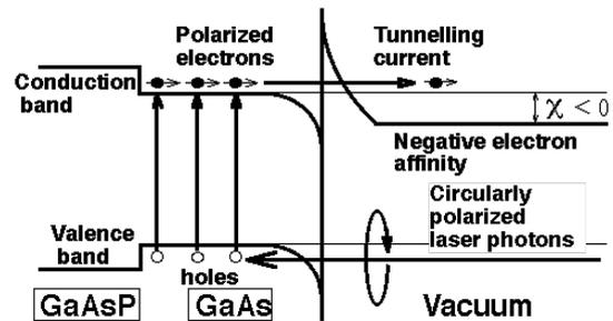
Fig. 1 : Principle of Strained GaAs-type PES
