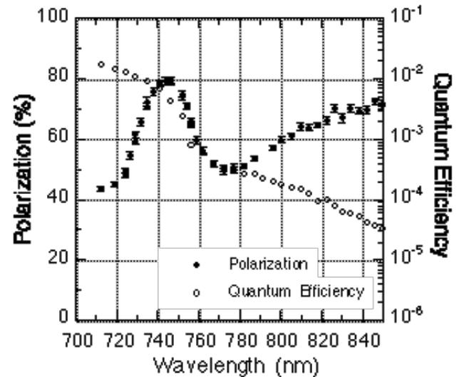
Fig. 3 : ESP and QE dependence on laser wave-length for SLSA#2 strained-layer superlattice PC.
