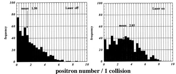
Fig. 5 Collision frequencies measured with acrylic Cerenkov counters for laser-on and laser-off.
