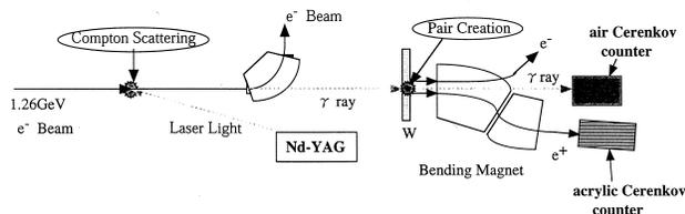
Fig. 3 Schematic illustration of an experimental system for generating polarized positrons..
