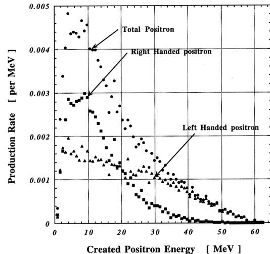
Fig. 2 Differential cross section of pair-creation as a function of created  $e^+$  energy for left handed  $e^+$ , right handed  $e^+$ , and total  $e^+$ .
