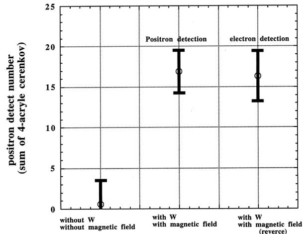
Fig. 6 Numbers of  $e^+$  pulse detected under the conditions : (a) Without a W-target and magnetic field, (b) With a W-target and magnetic field, (c) With a W-target and magnetic field (reversed current)
