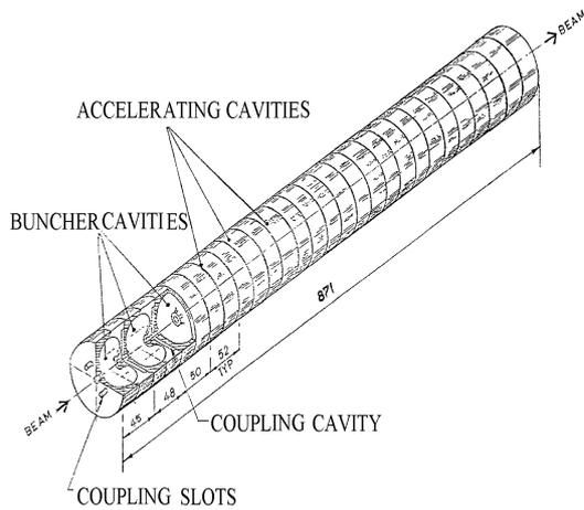
Fig.2 - On - Axis Coupled RF Linac
