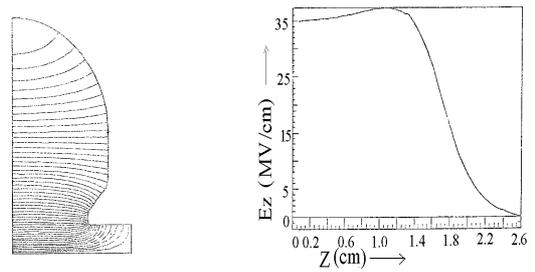
Fig. 4 - Electric field distribution and profile in the acceleration cavity
