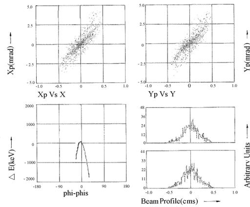
Fig.8-Phase Space, Intensity and Energy Distribution of the beam at the end of the Linac
