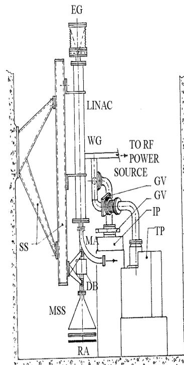
Fig.1 - RF Electron Linac
