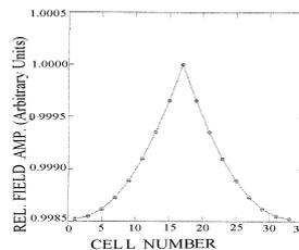
Fig.5 - Droop along the length of the cell
