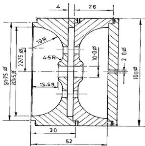
Fig.3-Acceleration Cavity for Cold Modelling and Testing
