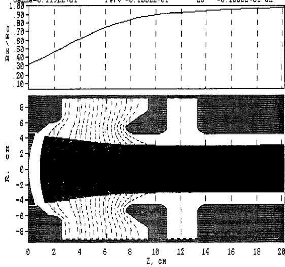
Figure 3: Modulation anode gun design of the klystron
