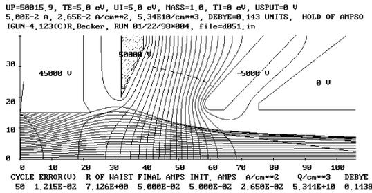
Fig. 3 The extraction electrodes and beam profiles in IGUN simulation.
