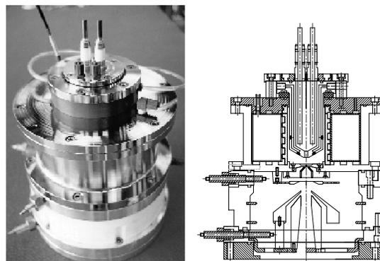
Fig. 1 A picture and a drawing of Duoplasmatron ion source.
