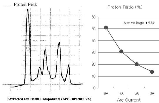
Fig. 6 Proton fraction measurements and their dependency on arc powers.
