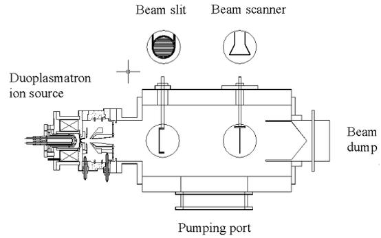
Fig. 4 Experimental setup of ion beam diagnostics.
