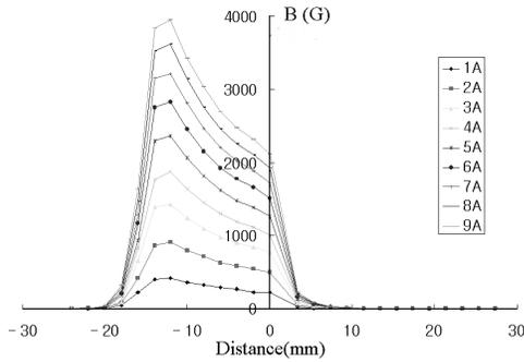
Fig. 2 Measured magnetic field strength between intermediate electrode and anode.
