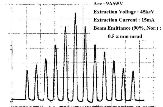
Fig.5 Beam emittance measured by multi-slit and beam scanner set.
