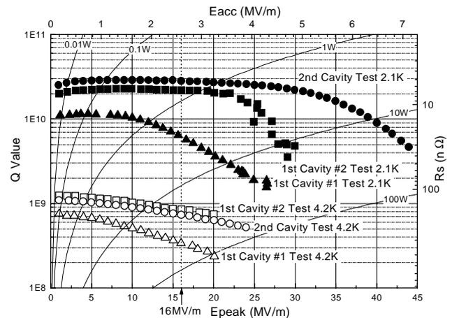
Fig. 3 Results of the performance tests for the two prototype cavities;  $Q$  values as a function of the surface peak electric field ( $E_{\text{peak}}$ )
