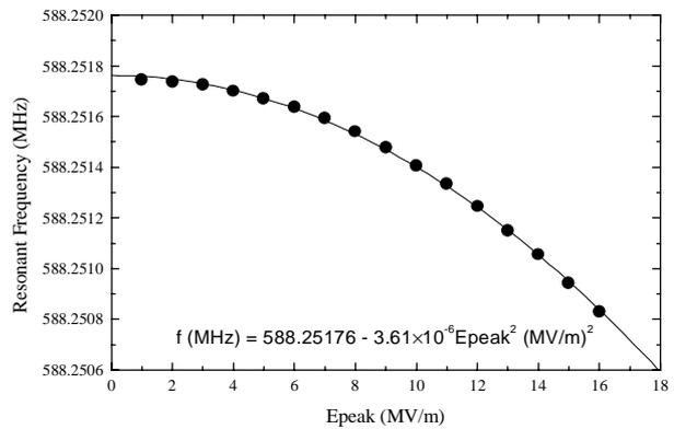
Fig. 5 Resonant frequency as a function of the surface peak electric field ( $E_{\text{peak}}$ )
