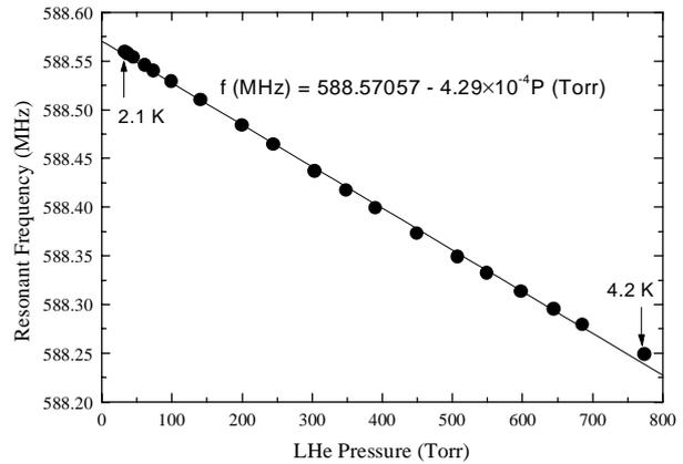
Fig. 4 Resonant frequency as a function of the pressure of the liquid helium
